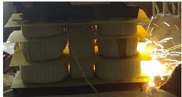
Fig.7. Fabricated model of arc welding machine
